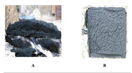
Figure 5. Intumesced plate exposed to fire with a dry film thickness of 1.5 mm for paint B. A) Side view; B) front view.
