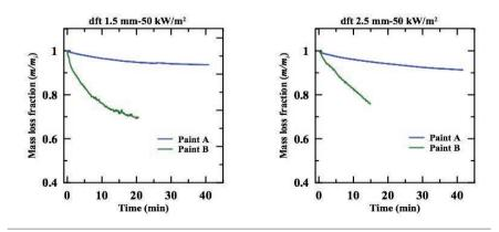
Figure 3. Comparison of mass loss fraction for different paints. dft, dry film thickness.
