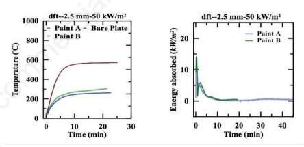
Figure 2. Variation of temperature and energy absorbed by Stainless Steel 310 plates for a dry film thickness of 2.5 mm. dft, dry film thickness.
