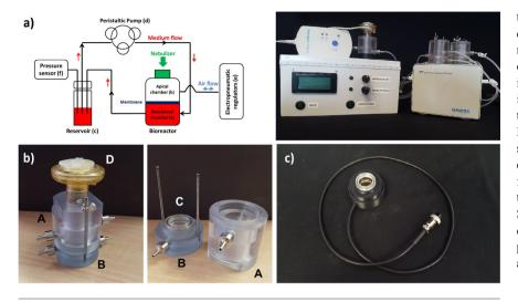
Figure 1. a) Schematic representation of the DALI system (on the left) and its picture (on the right); b) pictures of the component parts of the bioreactor; c) picture of the QCM device.
