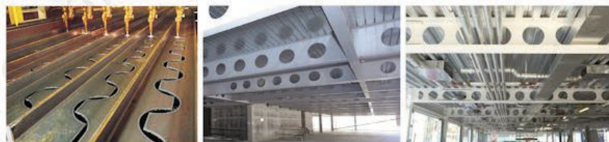
Figure 2. The cutting process of cellular beams.
