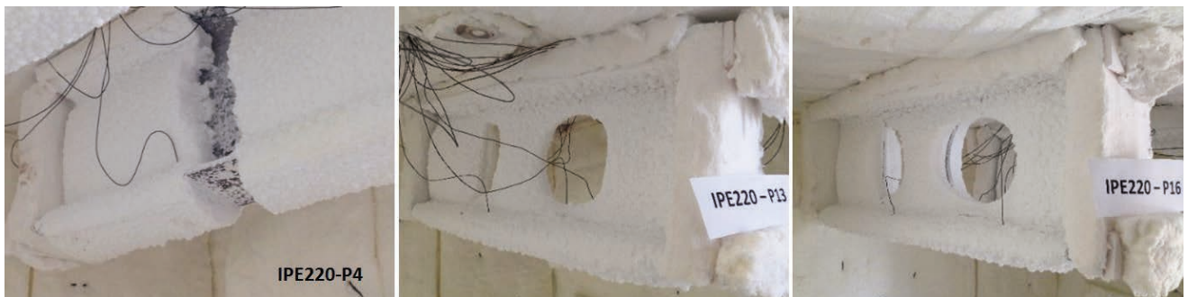
Figure 11. Intumescent coating expansion of test P4 (left), P13 (middle) and P16 (right) after test.
