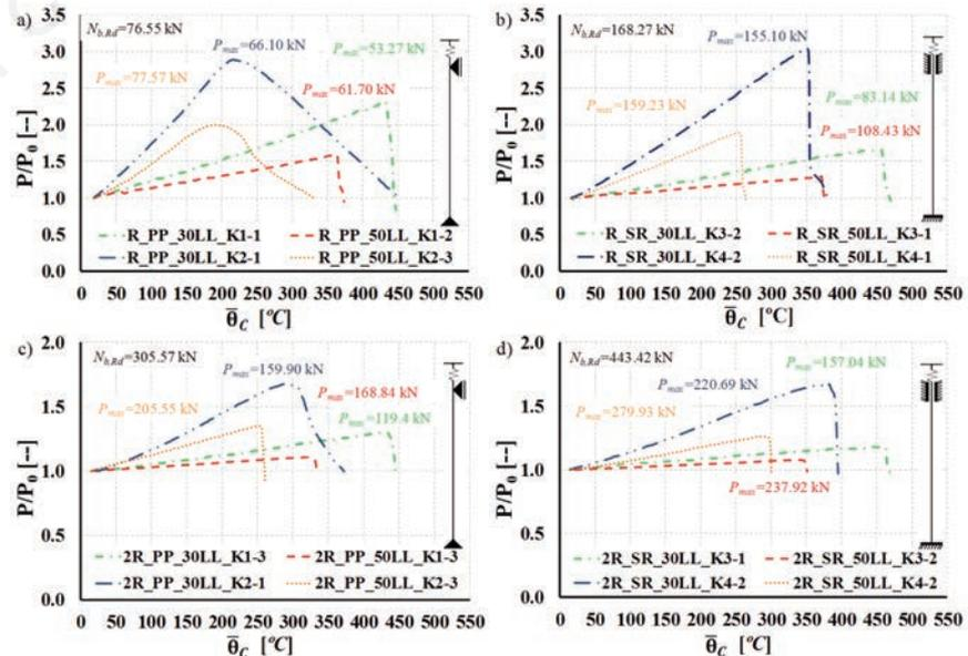
Figure 7. Non-dimensional restraining forces ratio for closed built-up cold-formed steel columns. a) R, pinned-end support; b) R, semi-rigid end support; c) 2R, pinned-end support; d) 2R, semi-rigid end support.
