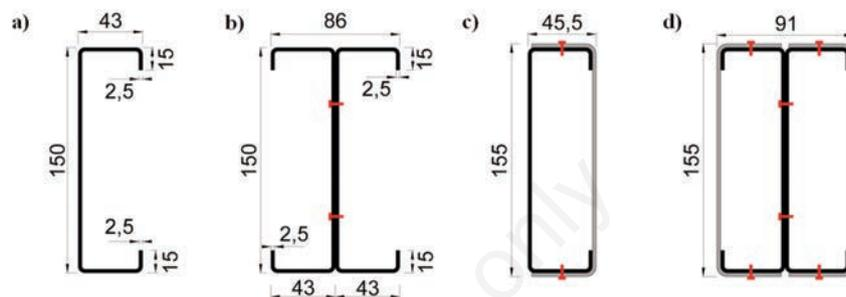
Figure 1. Dimensions of the cross-sections tested: a) C; b) I; c) R; d) 2R.
