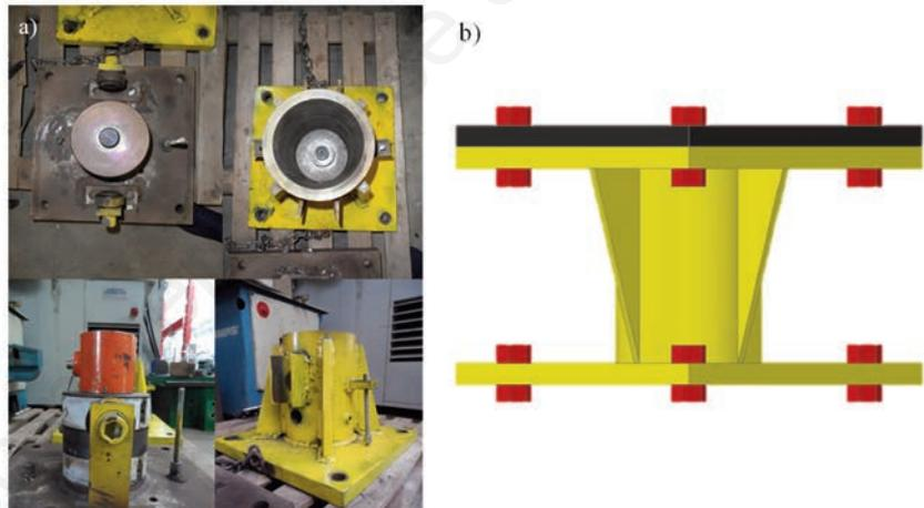
Figure 4. Device for measuring the restraining forces.
