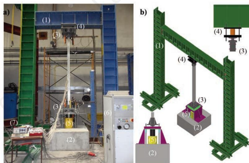
Figure 2. Experimental test set-up designed and built for the buckling tests. a) Test set-up; b) schema of the test set-up.
