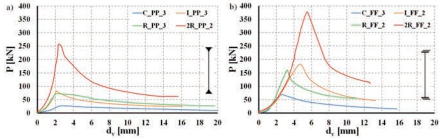
Figure 5. Load *vs* axial displacement diagrams for the compression tests undertaken on cold-formed steel columns with C, I, R and 2R cross-sections. a) Results for the pinned-end support condition; b) results for the fixed-end support condition.
