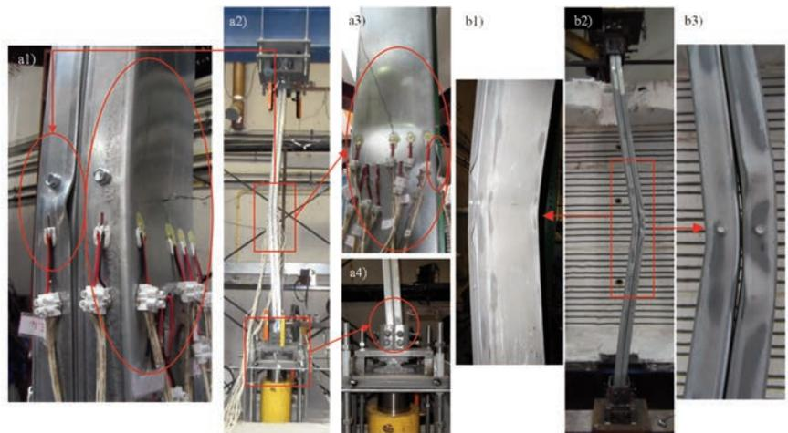
Figure 9. Failure modes observed for columns with closed built-up 2R cross-section and fix-ended support condition. a) Buckling tests at ambient temperature; b) fire tests with restraint to thermal elongation.
