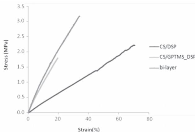
Figure 4. Stress-strain curves of chitosan/dibasic sodium phosphate (CS/DSP), chitosan/ $\gamma$ -glycidoxypropyltrimethoxysilane\_dibasic sodium phosphate (CS/GPTMS\_DSP), and bi-layer flat membranes tested in wet state.
