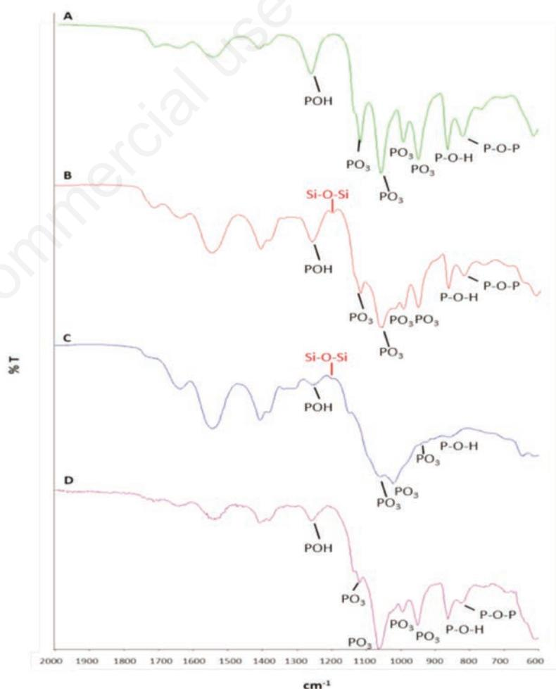
Figure 2. Fourier transform-infrared spectroscopy-attenuated total reflectance spectroscopy spectra of chitosan/dibasic sodium phosphate (A), chitosan/ $\gamma$ -glycidopropyltrimethoxysilane\_dibasic sodium phosphate (B), external (C) and internal side (D) bilayer membrane.
