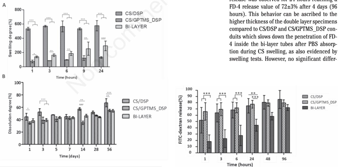
**Figure 5.** Swelling (A) and total dissolution (B) percentages of chitosan/dibasic sodium phosphate (CS/DSP), chitosan/ $\gamma$ -glycidopropyltrimethoxysilane dibasic sodium phosphate (CS/GPTMS\_DSP), and bi-layer flat membranes in phosphate buffer solution as a function of time. Column heights correspond to the mean values. Bars indicate standard deviations ( $n=3$ ). \* $P < 0.05$ , \*\* $P < 0.01$ , \*\*\* $P < 0.001$ .
