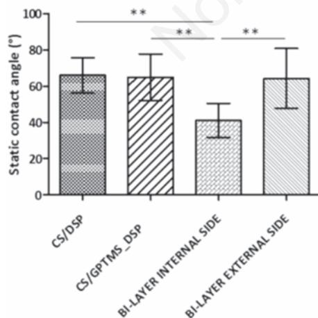
Figure 3. Static water contact angle of chitosan/dibasic sodium phosphate (CS/DSP), chitosan/ $\gamma$ -glycidoxypropyltrimethoxysilane\_dibasic sodium phosphate (CS/GPTMS\_DSP), internal and external side of bi-layered film samples. Histograms reported the average values and the standard deviations.  $**P < 0.01$ .
