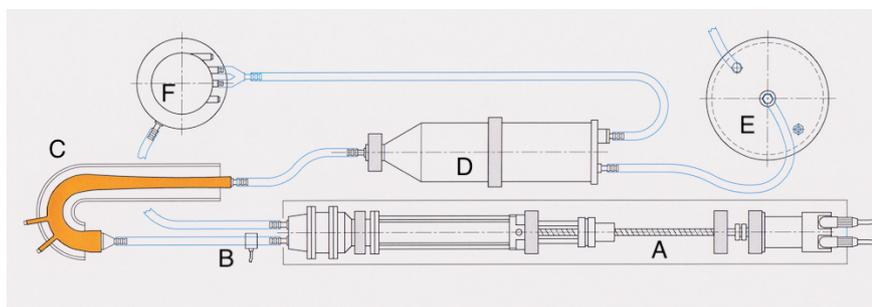
Figure 1. Schematic representation of the pulsatile system. A, pump; B, flow meter; C, *ex-vivo* porcine aortic specimen; D, resistance chamber; E, windkessel compartment; F, water reservoir.
