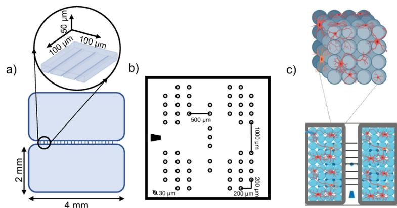
Figure 1. Sketch of the *in vitro* model: a) PDMS mask details; b) MEA-4Q active area configuration; c) 3D cell cultures made up of glass microbeads.
