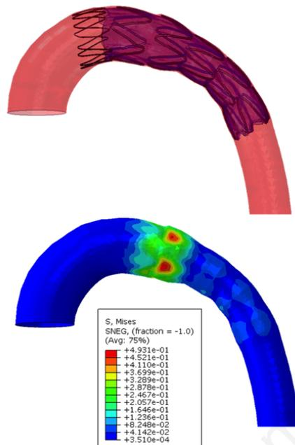
Figure 2. Distribution of Von mises stress induced by stent-graft deployment.
