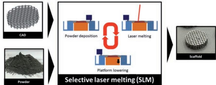
Figure 1. Schematic representation of selective laser melting process.
