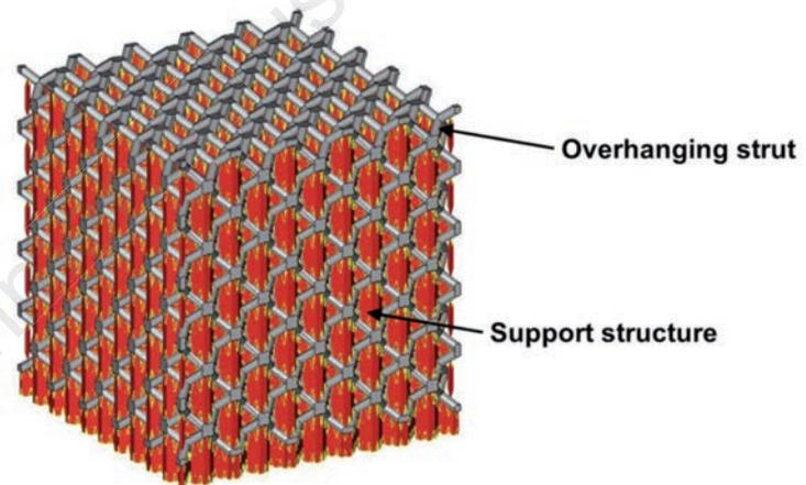
Figure 2. Overhanging struts and support structures for metallic scaffolds.
