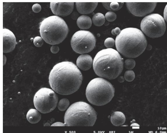
Figure 3. Morphology of powder used in selective laser melting.
