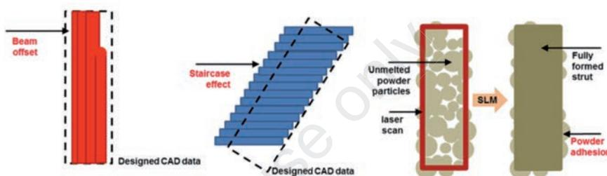
Figure 5. Causes of inaccuracy of production of the designed lattice structures by selective laser melting.
