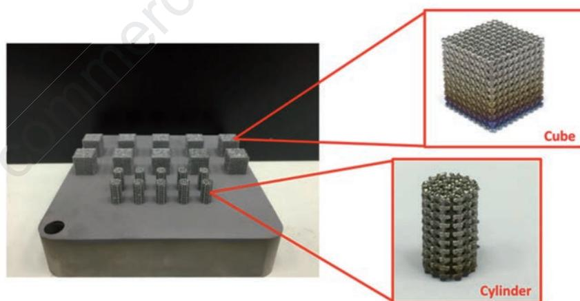
Figure 6. Compression test coupons fabricated by selective laser melting.
