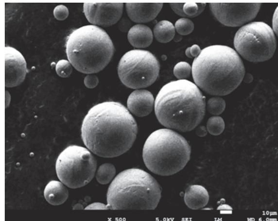
Figure 3. Morphology of powder used in selective laser melting.
