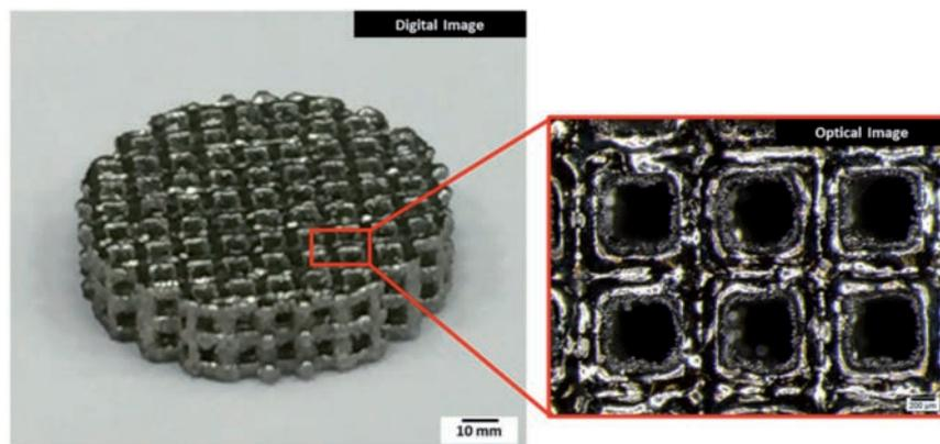
Figure 4. Metallic scaffold fabricated by selective laser melting: overall scaffold (digital image, left) and its magnification (optical image, right).
