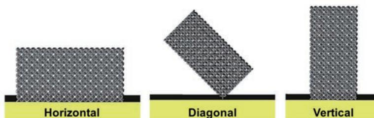
Figure 7. Build orientations of lattice structures in selective laser melting.
